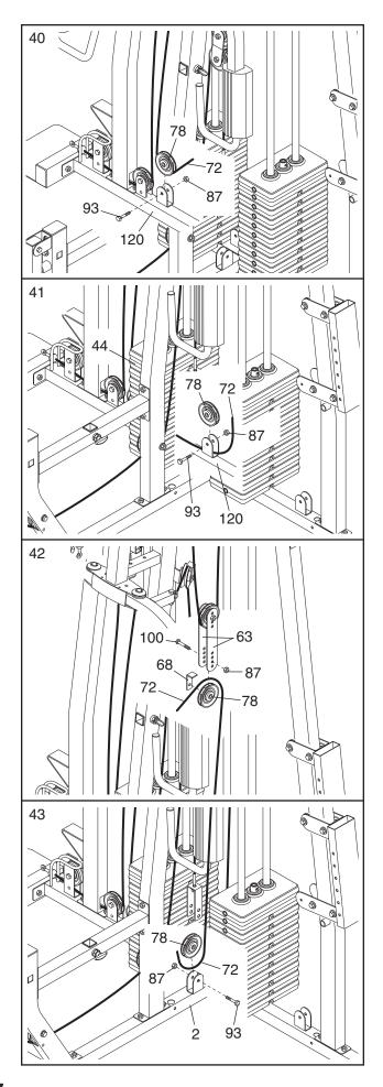
44. Wrap the VKR Low Cable (72) over a 3 1/2" Pulley (78). Attach the Pulley and a Cable Trap (68) between the lower set of holes in the "U"-bracket (64) with a 3/8" x 2" Bolt (100) and a 3/8" Nylon Locknut (87). Make sure that the Cable Trap is turned to hold the Cable in the groove of the Pulley.
